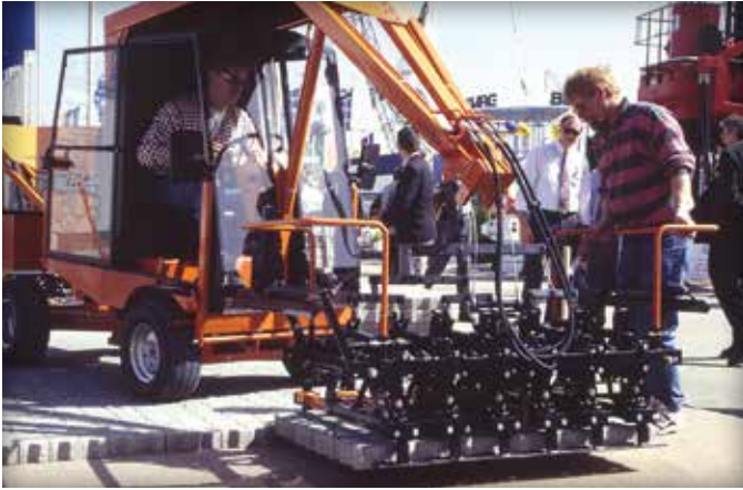
Figure 3. Motorized equipment with a mechanical clamp.
