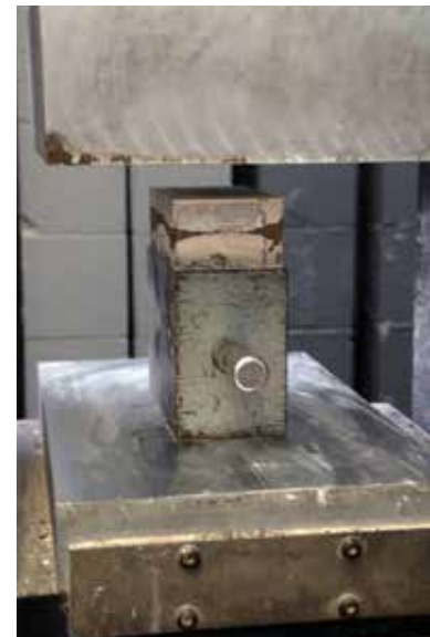
Figure 1. A concrete paver capped on the top and bottom with gypsum and positioned in a compressive strength machine for testing.
