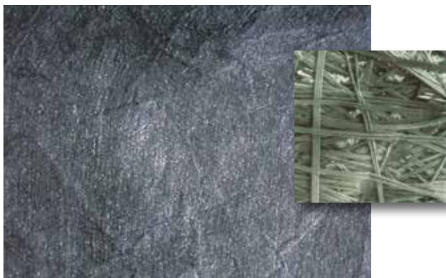
Figure 15. Non-woven heat bonded geotextile with close-up
