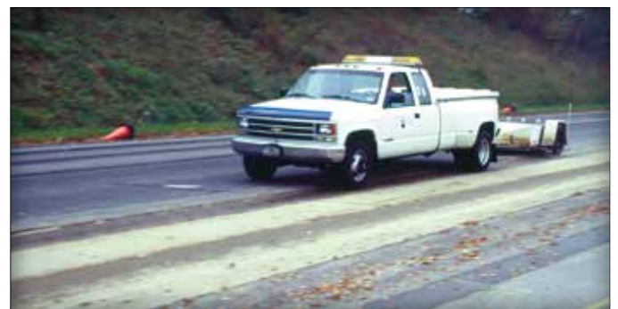
Figure 4. ASTM E 274 Test Equipment consists of a truck and trailer assembly. A tire within the trailer is towed at a given speed, locked, and skidded across water dispensed on the pavement in front of it.
