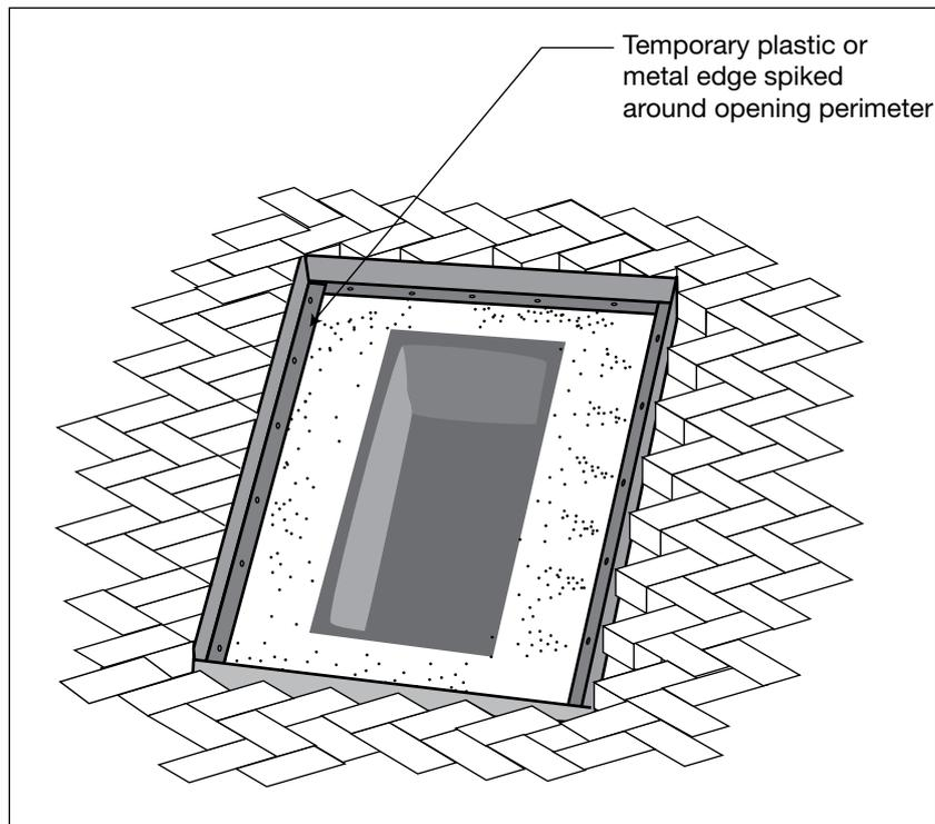
Figure 9. Temporary bracing at the pavement opening will help keep units in place during excavation, repairs and reinstatement.
