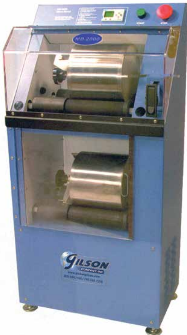
Figure 1. The Micro-Deval test apparatus. Source: Gilson Company
