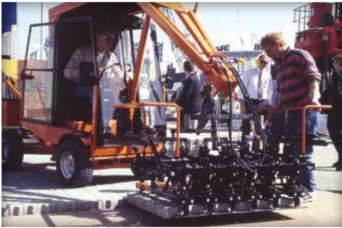
Figure 3. Motorized equipment with a mechanical clamp.
