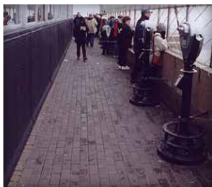
Figure 1. Concrete pavers provide a durable and attractive roof plaza deck surface. At left is the observation deck on the 86 th floor of Empire State Building in New York City. At center is a hotel plaza deck constructed with concrete paving slabs.
