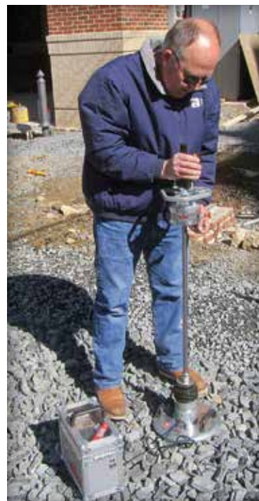
Figure 22. Testing base stiffness using light-weight deflectometer.
