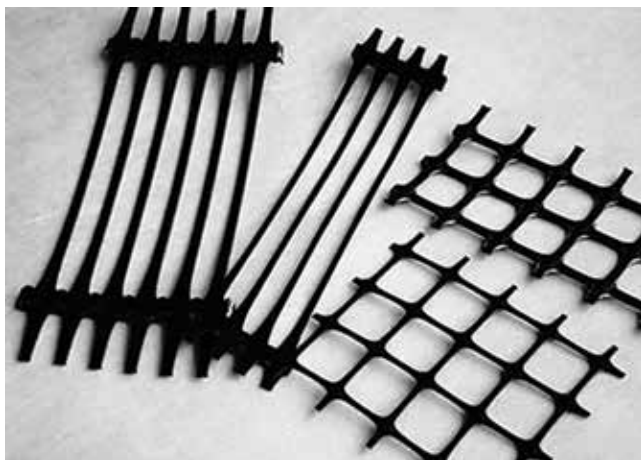
Figure 20. Uniaxial and biaxial, punched and drawn geogrids
