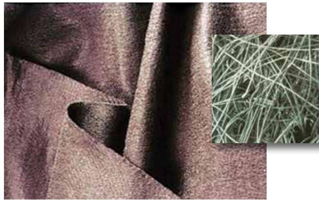
Figure 14. Non-woven needle punched geotextile with close-up
