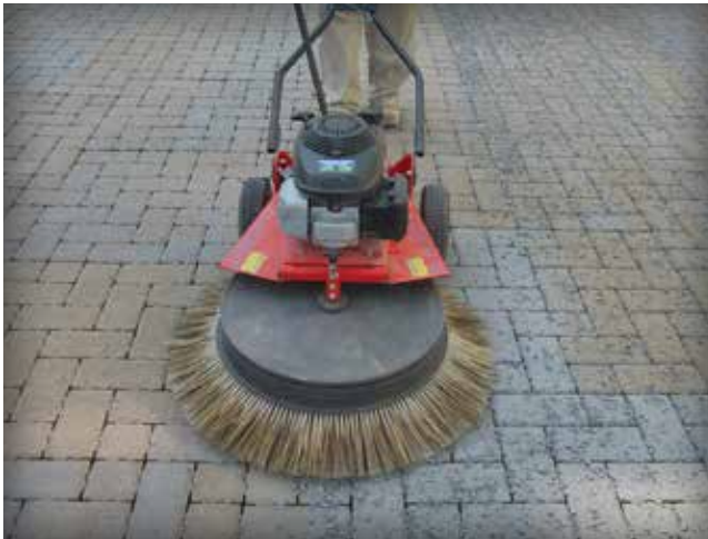
Figure 16. Rotary brushes increase cleaning efficiencies.
