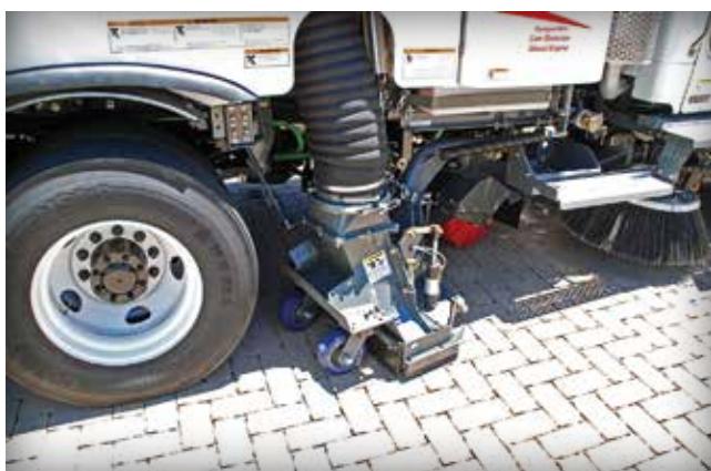
Figure 22. A true vacuum machine cleaning neglected PICP.
