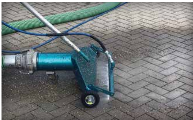
Figure 23. This equipment provides combined washing and vacuum of unmaintained PICP.
