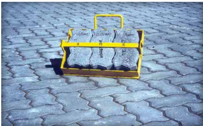
Figure 16. A simple gauge for checking dimensional tolerances on the job site.
