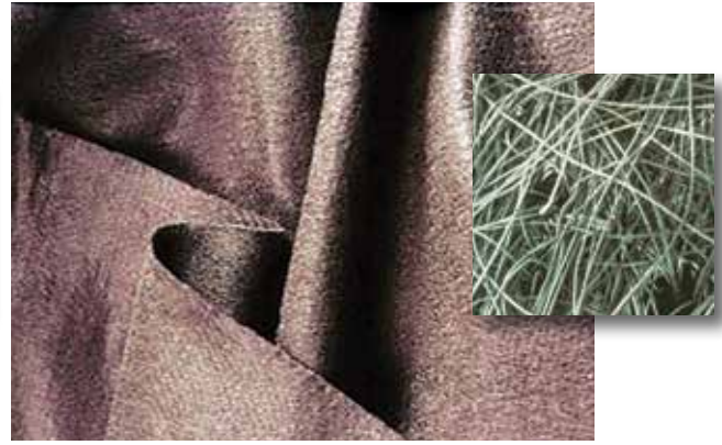
Figure 14. Non-woven needle punched geotextile with close-up
