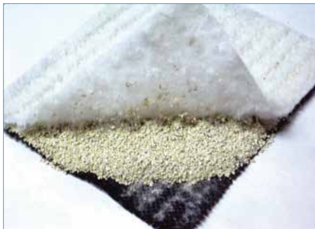
Figure 6. Geosynthetic clay liners
