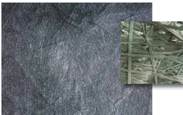
Figure 15. Non-woven heat bonded geotextile with close-up
