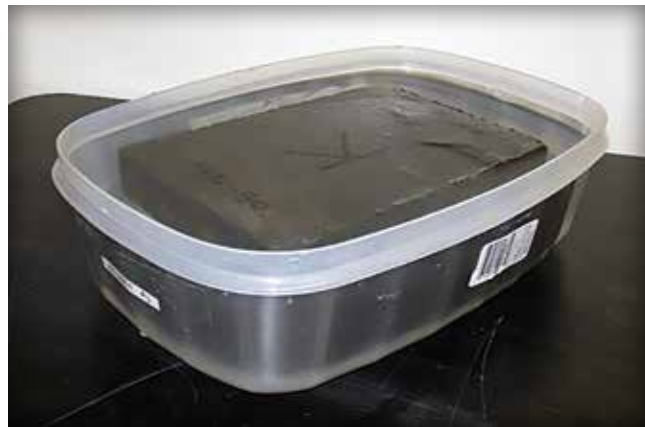
Figure 3. Test specimen from a slab immersed in a 3% saline solution ready for exposure to laboratory freeze-thaw cycles.
