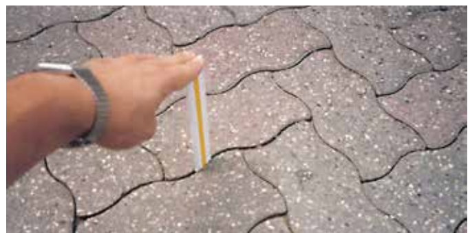
Figure 2. Refill joints with dry masonry sand if loss is greater than \frac{1}{2} in. (12 mm).
