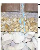
→ 3 1/8 in. (80 mm) thick pavers with permeable joints
