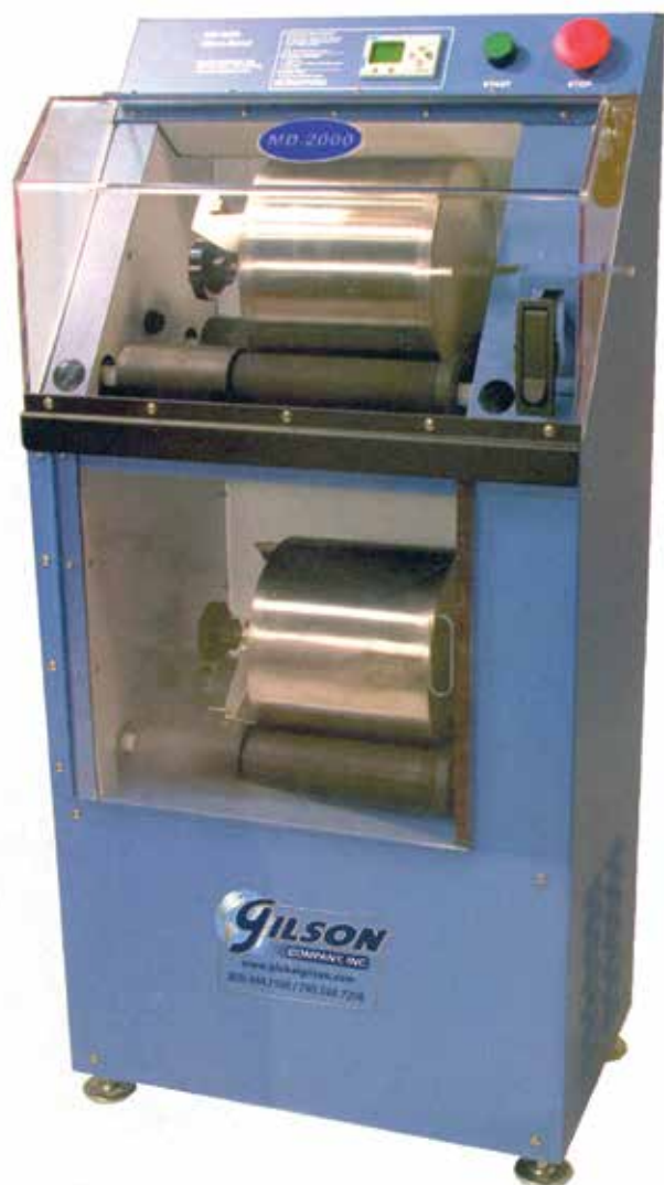
Figure 1. The Micro-Deval test apparatus. Source: Gilson Company
