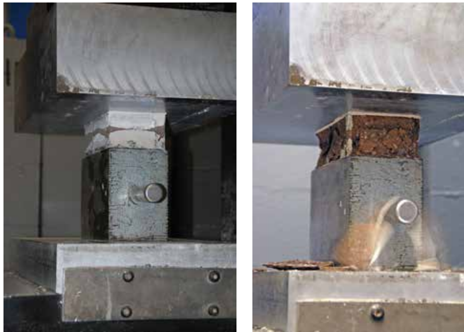
Figure 6. Left: a capped concrete paver under load in a compression testing machine; Right: a paver tested in compression; the moment it breaks is the recorded load.
