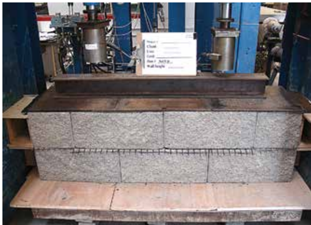
Figure 19. Geogrid connection testing with SRW units
