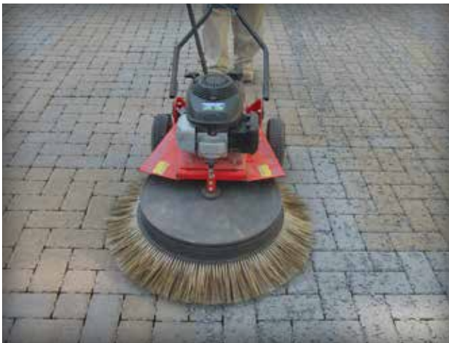
Figure 16. Rotary brushes increase cleaning efficiencies.
