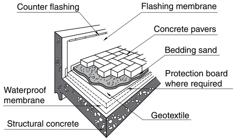
Figure 3. Roof assembly
