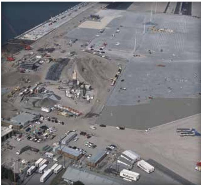
Figure 14. The Port of Oakland, California, is the largest mechanically installed project in the western hemisphere at 4.7 million sf (470,000 m<sup>2</sup>).
