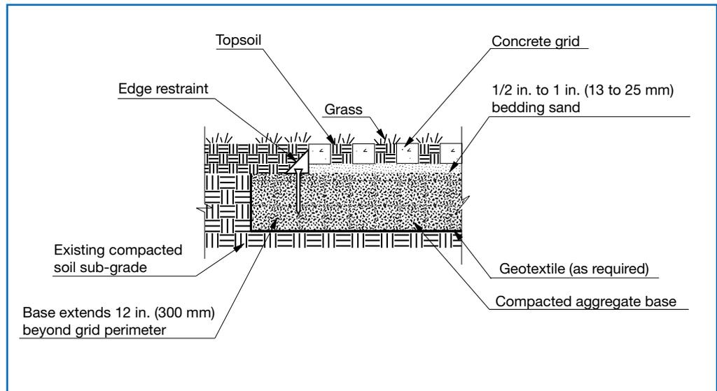
Figure 15. Typical concrete grid pavement over dense-graded base
