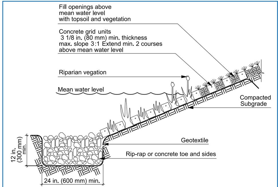
Figure 19. Lake side stabilization with concrete grids
