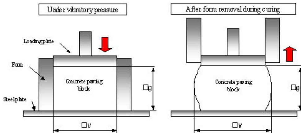
Figure 2. Plastic deformation.
