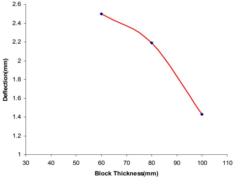
Figure 7. Effects of block thickness on behavior of block pavement
