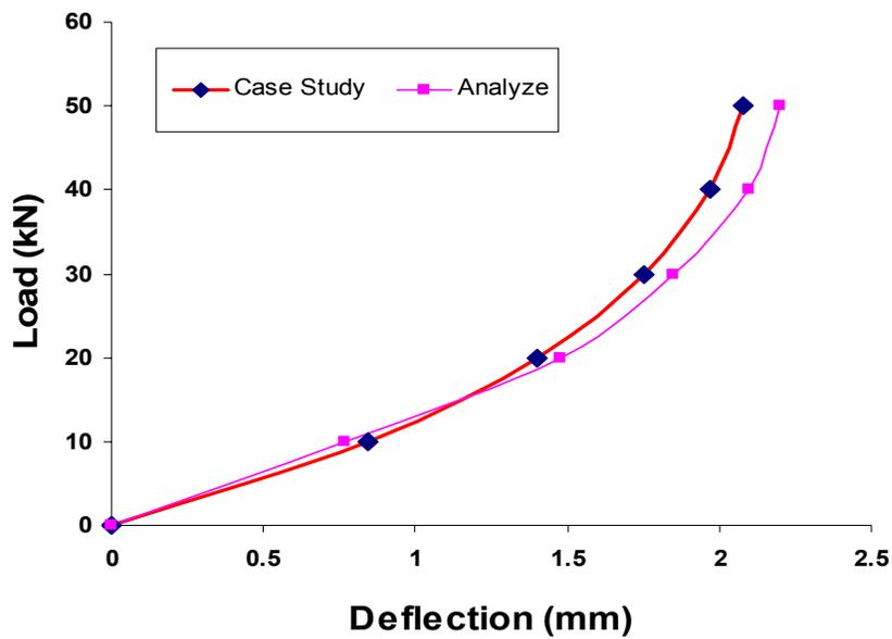
**Figure 3. Deflection of pavement against increasing load for the finite element model and cues study**
