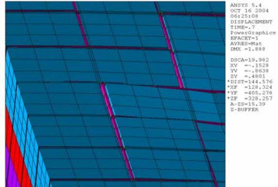
**Figure 10. Rotation of blocks for development of interlocking in herringbone patterns**
