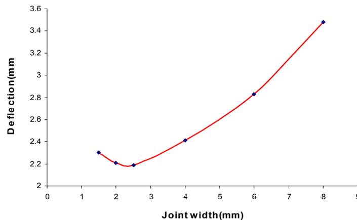
**Figure4. Pavement deflections with varying joint width**
