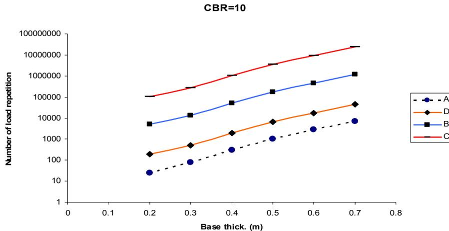
**Figure11. Typical design chart; E Block = 4,200MPa, E bound base = 35,000 MPa, Block Thickness = 80 mm**
