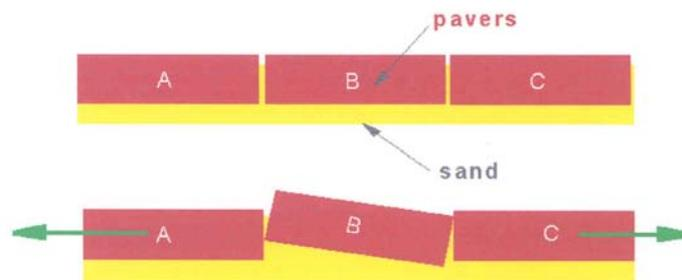
Figure 8. Rotation of Paver B causing outward wedging of Pavers A and B (Shackel, 2003)
