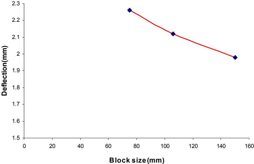
**Figure 5. Effect of block size (consistent 80 mm thickness) on deflection behavior of block pavement**
