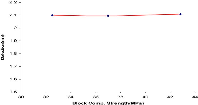
**Figure 6. Effect of block compressive strengths on behavior of block pavement**
