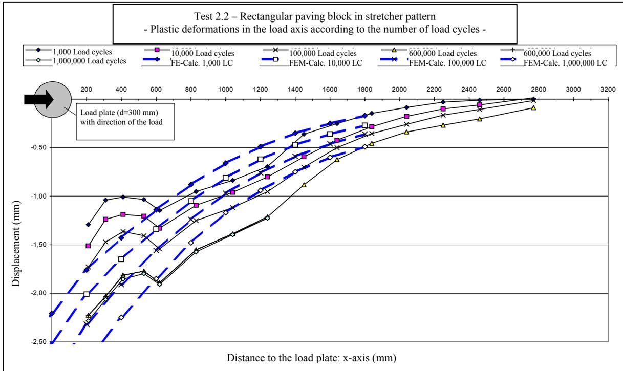
Figure 5. Laboratory test results (thin lines) versus results of numerical simulations (dashed line)
