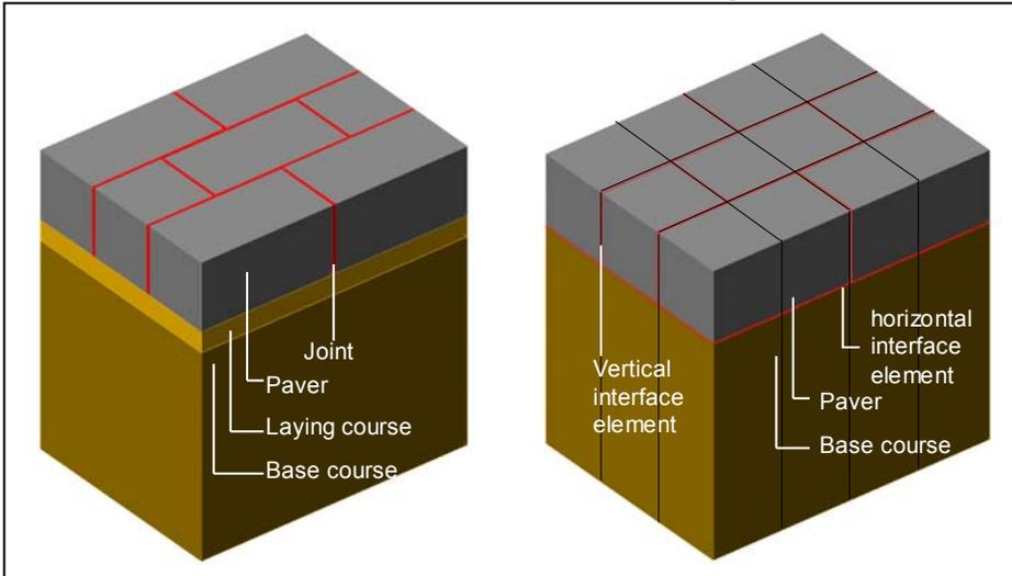
**Figure 4. Block pavement model (Ascher 2003)**
