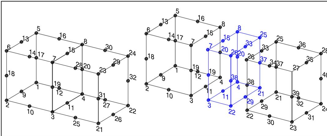
Figure 2. Coupled 20-node elements, left: rigid coupling, right: flexible coupling (Ascher 2003)
