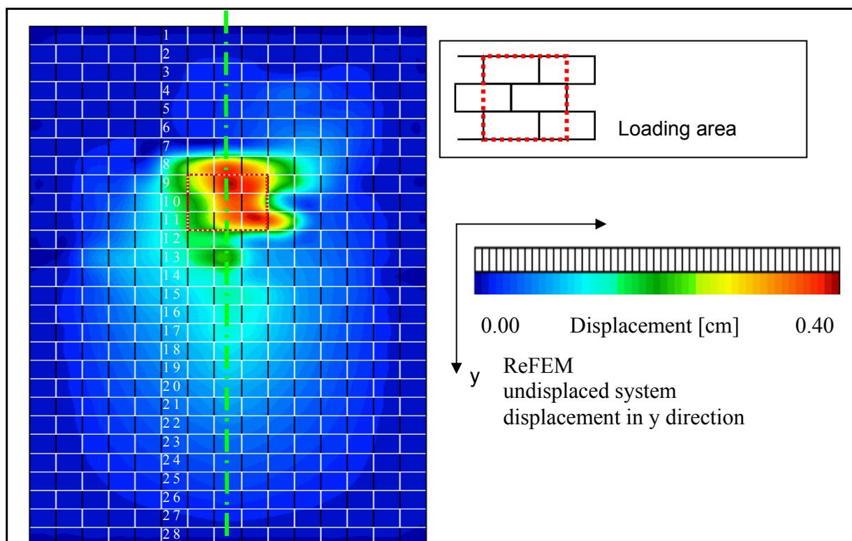
**Figure 6. Results of the numerical simulation for the stretcher pattern**
