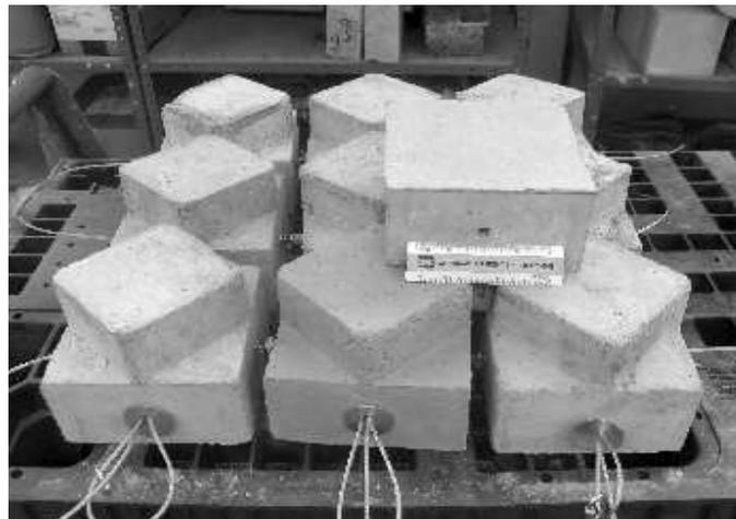
**Figure 5. Nine-block array with an additional block fitted into the opening on the upper surface. Test array is assembled with a clamp cable arrangement to allow the effect of block spacing to be evaluated.**
