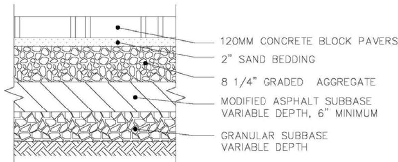
**Figure 4. Seagirt Generalized Pavement Design (1" = 25 mm)**
