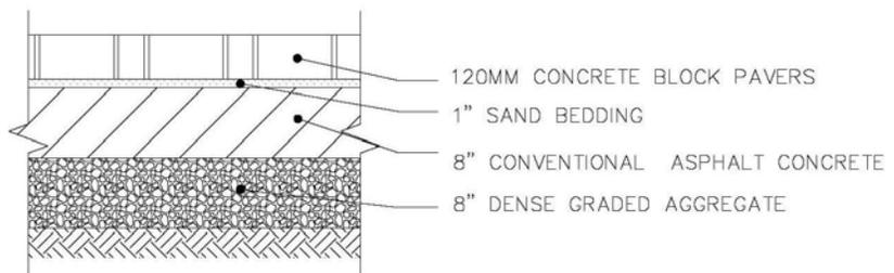
**Figure 9. WWL Pavement Section (1" = 25 mm)**
