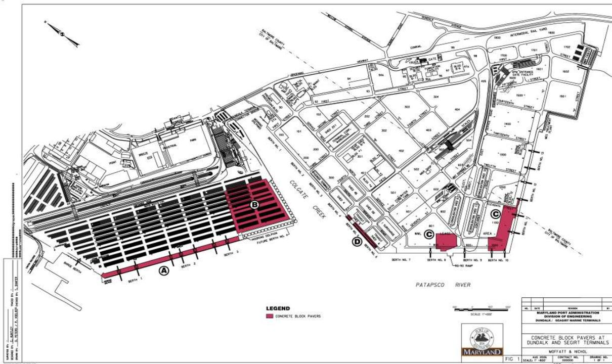
Figure 1. Concrete Paver Block Pavements at DMT and SMT
