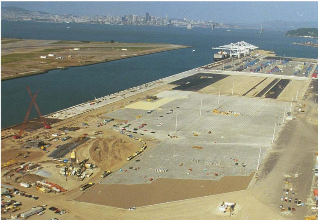
**Figure 1. Completion of 470,000 m<sup>2</sup> of interlocking concrete pavement at the Port of Oakland, California, in March 2002**
